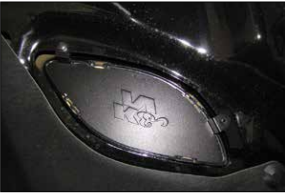
28. Place the provided block off into position and reinstall the factory screws. NOTE: On models with out the two screws holding the grill, insert the block-off like a grommet into the opening. NOTE: This block off does not seal the heat extractor vent completely. It is intended to reduce the amount of moisture that can directly come in contact with the air filter.
