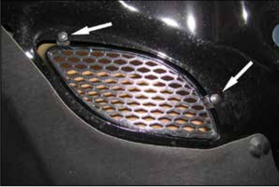
27. Some Dodge Durango models may be equipped with heat extractor vents in the hood. During inclement weather or driving in wet conditions, K&N® recommends installing the provided heat extractor block off plate. Remove the two screws that secure the factory grid in position. NOTE: Some model may not have the screws holding in the grill.
